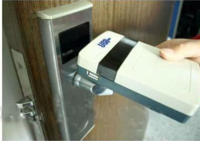
collect opening records from hotel lock
