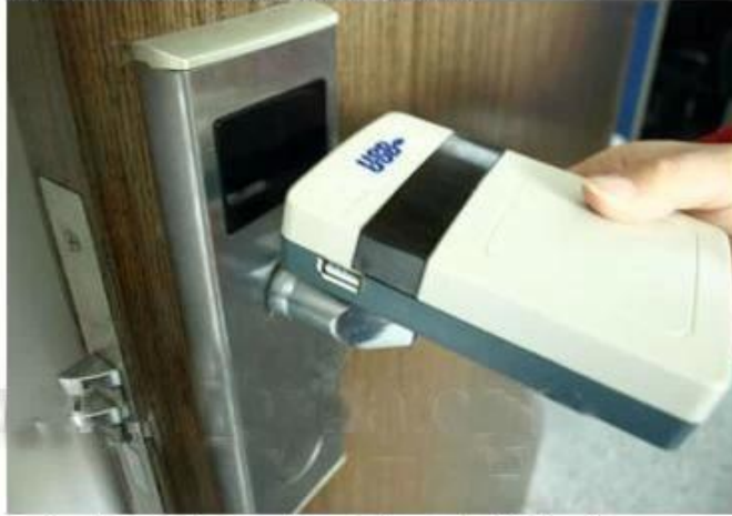
collect opening records from hotel lock
