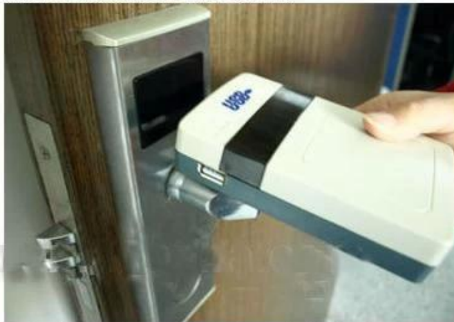
collect opening records from hotel lock
