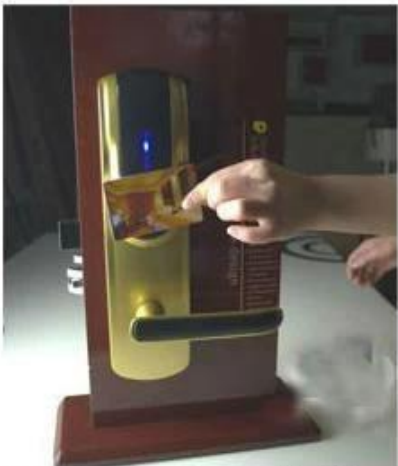
opening the door with RF card
