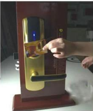
opening the door with RF card
