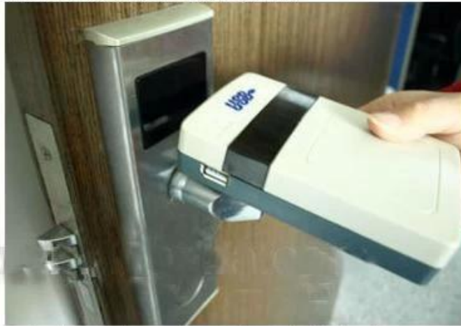
collect opening records from hotel lock
