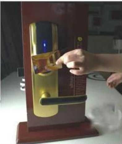
opening the door with RF card
