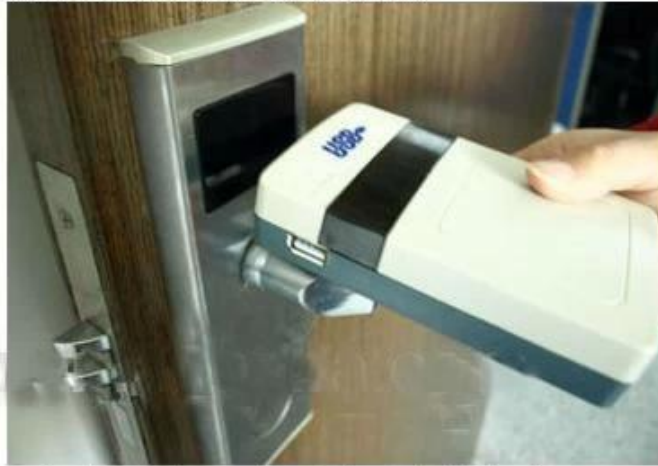
collect opening records from hotel lock
