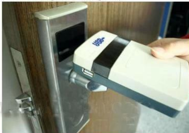
collect opening records from hotel lock
