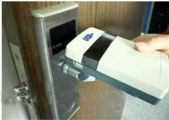
collect opening records from hotel lock
