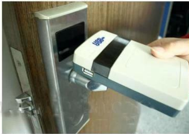
collect opening records from hotel lock
