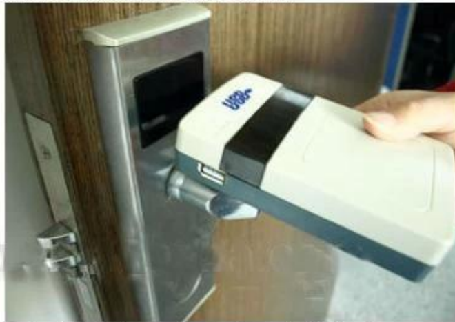
collect opening records from hotel lock
