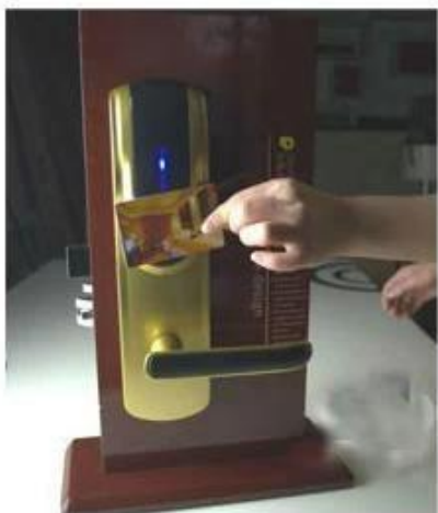
opening the door with RF card
