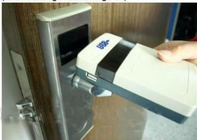
collect opening records from hotel lock
