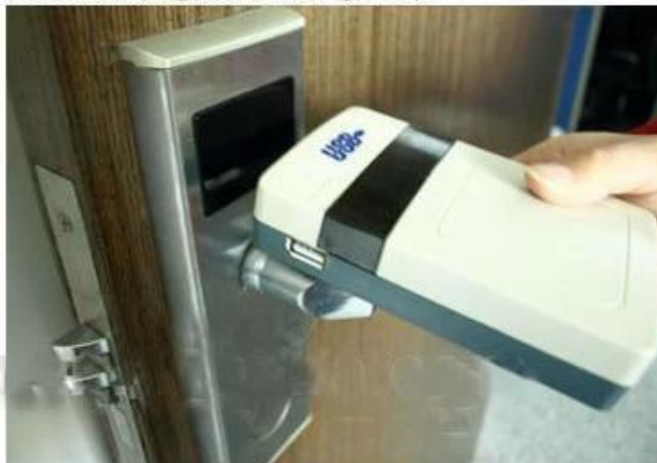
collect opening records from hotel lock
