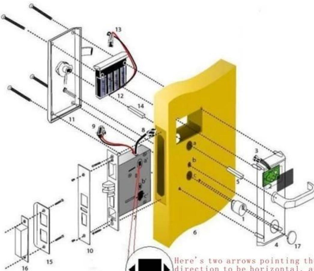
Here's two arrows pointing the direction to be horizontal, and the lock cylinder cover on the upper, non-vertical point!
