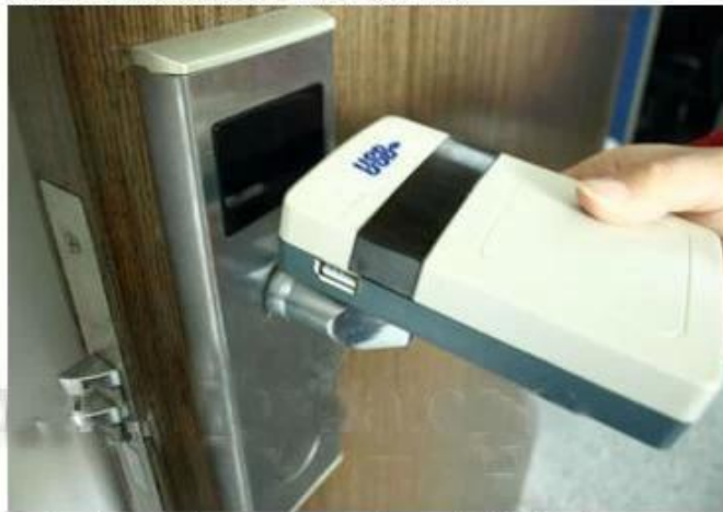
collect opening records from hotel lock
